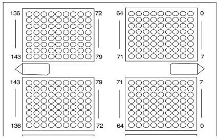
FIGURE 2-12. Unbalanced Digital Audio/Digital Video Input Connector Matrix
