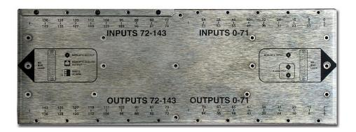
FIGURE 4-24. Redundant Midplane
