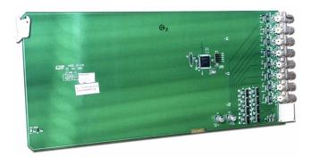
FIGURE 4-1. SD Video Input Board
