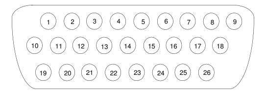
FIGURE 2-15. DB-26 High-Density Male Connector
