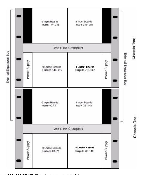
FIGURE 1-5. 288x288 SD/HD Chassis (non-expandable)
