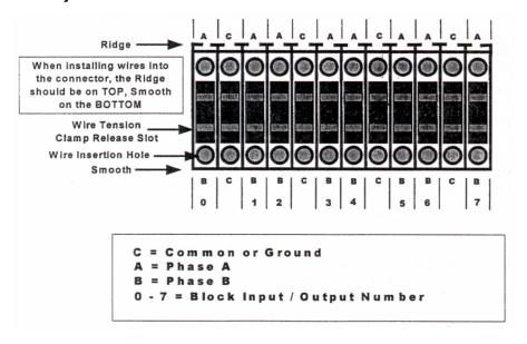
FIGURE C-2. Tension Clamp Connector (viewed from the back)
