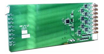
FIGURE 4-8. SD Output Board
