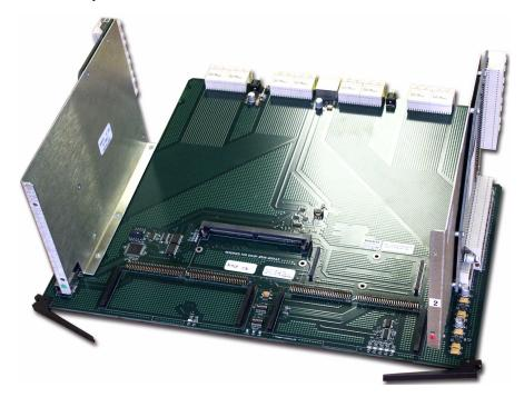
FIGURE 4-22. Output Buffer card
