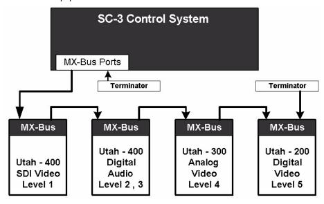
FIGURE 2-7. Block Diagram of the MX-Bus Daisy Chain.
