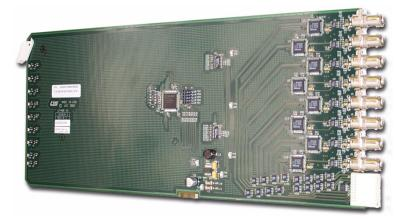
FIGURE 4-9. SD (Multi-Rate)Output Board
