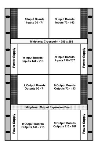
FIGURE 1-3. The Utah-400 288 x 288 Router Configuration
