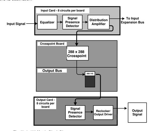
FIGURE 1-1. The Utah-400 Matrix Block Diagram
