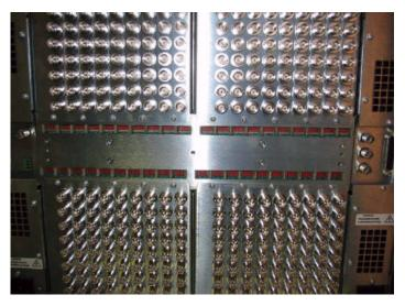
FIGURE D-5. Utah-400 Frame with Expansion Port cover removed
