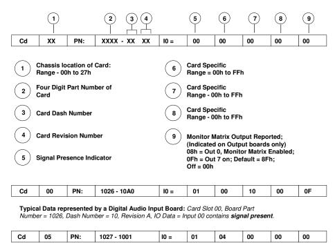
Typical Data represented by a Digital Audio Output Board: Card Slot 05, Board Part Number = 1027, Dash Number = 10, Revision 01, IO Data = Output 00 contains signal present.
