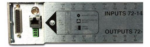
FIGURE 4-25. Audio Midplane's RJ-45 connection
