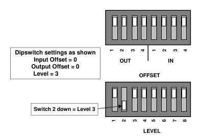
FIGURE 2-10. Utah-400 Configuration Dipswitches as they appear on the Crosspoint Carrier Board
