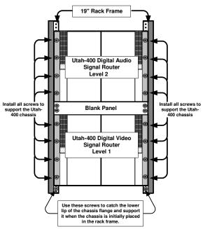
FIGURE 2-2. Utah-400 Chassis Mounted in 19" Rack Frame
