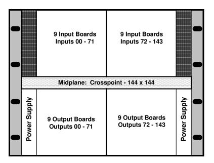
FIGURE 1-2. The Utah-400 144 x 144 Configuration
