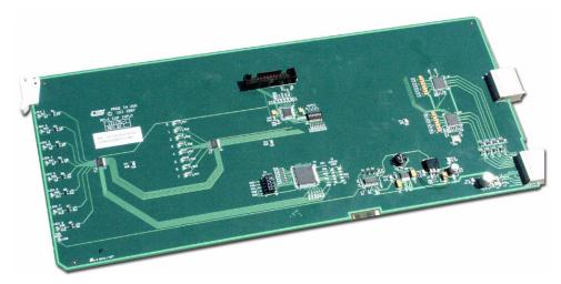
FIGURE 4-6. Reclocking Input Expansion card
