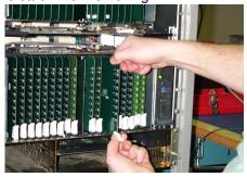
FIGURE 3-2. Input/Outut Board Replacement and Removal
