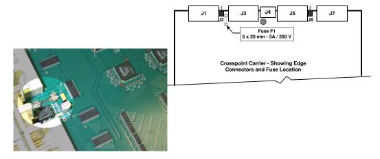
FIGURE 4-35. Crosspoint board fuse assembly
