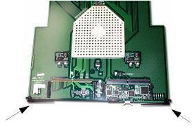
FIGURE 3-3. Crosspoint Board Replacement and Removal
