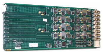
FIGURE 4-3. Analog to Digital Board
