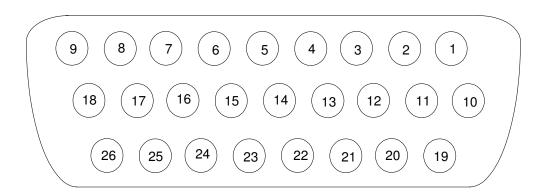
FIGURE 2-16. DB-26 High-Density Female Connector
