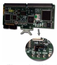
FIGURE 4-21. Video crosspoint module jumper location
