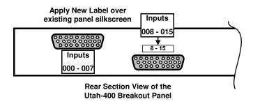
FIGURE C-3. Breakout Panel Label Application
