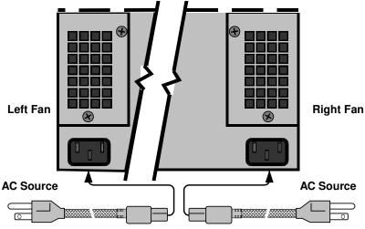
FIGURE 2-17. Utah-400 Power Connections
