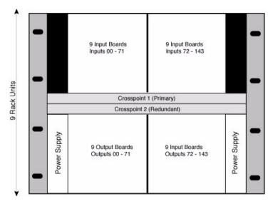
FIGURE 1-4. 144x144 with Redundant Crosspoints
