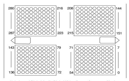
FIGURE 2-13. Unbalanced Digital Audio/Digital Video Output Connector Matrix
