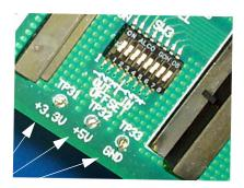
FIGURE 4-36. Audio Crosspoint board test points
