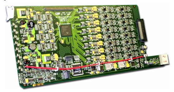
FIGURE 4-32. DAC Output Module
