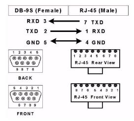
FIGURE B-1. Debug Port Cable Pinouts
