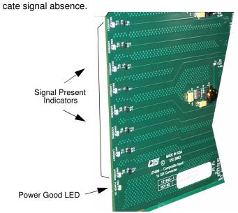
FIGURE 4-5. Analog to Digital card LEDs
