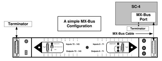
FIGURE 2-6. The MX-Bus Installation to an SC-3 Controller
